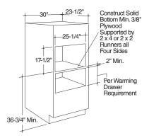
Additional clearances between the cutouts may be required. Check to be sure the oven supports above the warming drawer do not obstruct the required interior depth and height. See warming drawer installation instructions for details.
