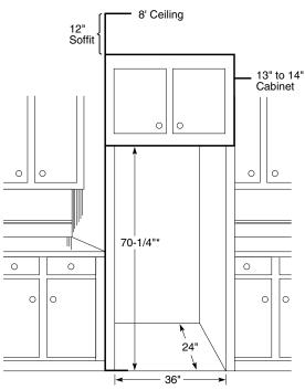
\*The rough-in dimension of 70-1/4" is minimum and is measured from the finished floor to top of opening (or the underside of the overhead cabinets). For Models with Tim Kit: If frameless style cabinets are planned for above the refrigerator, you may need to consider adding a maximum of 1/4" (70-1/2") to height of opening to allow additional clearance between cabinet doors and top of refrigerator trim when cabinet doors are in open position.
