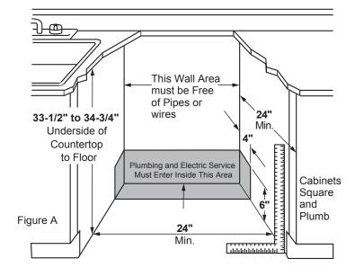
**NOTE:** Dishwasher must not be installed more than 10 feet from sink for proper drainage. All plumbing and electrical work must be in accordance with local codes. Dishwasher includes drain hose and leveling legs.
