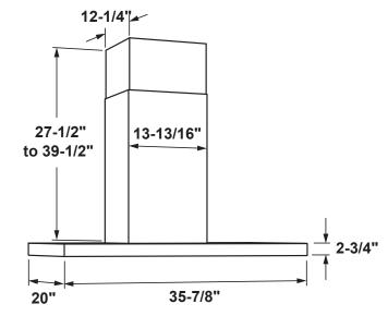
36" models require a 36"-wide opening \*The supplied duct cover fits 7'-7" to 9'-6" ceiling heights (10' ceiling height with optional high ceiling kit UX10DC83SS)
