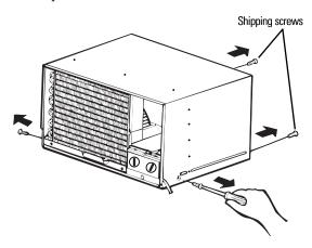
Slide the air conditioner from the case by gripping the base pan handle and pulling forward while bracing the case.
