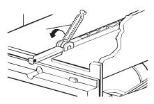
Attach the front grille to the case by inserting the tabs on the grille into the slots on the front of the case. Push the grille in until it snaps into place.
