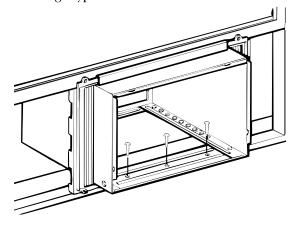
Pull the accordion panels to each window sash track. Attach them on each side to the window sash and the window stool using 4 type C screws.
