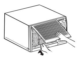
Clean the filter with warm, soapy water. Rinse and let the filter dry before replacing it.
