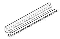
Install the top mounting rail with 3 type A screws on the inside of the case. Insert the frames for the accordion panels into the top mounting rail and the frame guides. Attach the accordion panels to the side of the case using 5 type A screws.
