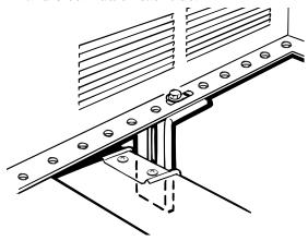
Adjust the carriage bolts and the lock nuts in each support so that the case is installed with a slight tilt to the outside. Use a level; about 1/3 bubble will be the correct case slant to the outside. Tighten the bolts.
