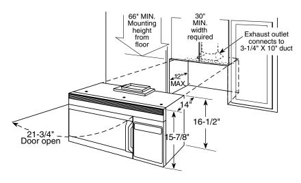
**Important Information:** When installing the Counter Saver Plus<sup>™</sup> microwave oven over a range, allow minimum of 2" from bottom of Counter Saver Plus<sup>™</sup> microwave oven to top of range backguard to allow for removal of light covers.
