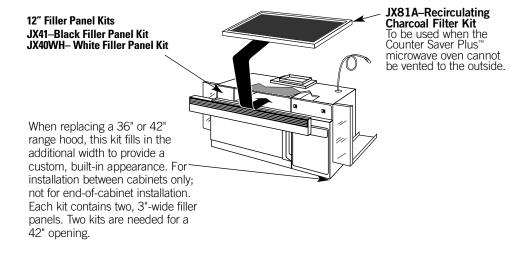
**Ventilation Options:** The Counter Saver Plus™ microwave oven is designed for adaptation for the following three types o ventilation:
