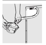
If the sink is 34" or higher from the floor, the excess water in Unicouple hoses cannot be drained directly into the sink. It will be necessary to drain excess water from hoses into a bowl or suitable container that is held outside and lower than the sink.
