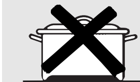
Pans with rounded, curved, ridged or warped bottoms are not recommended.
