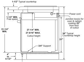
Add suitable filler to match adjacent cabinets when needed to maintain toe kick alignment Side View
