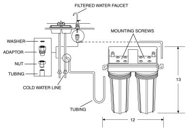
Note: Can be installed undercounter (as shown), in basement, or other convenient location. See installation instructions packed with product for complete details.
