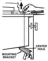
Choose the mounting bracket with the center hole. Hang the bracket from the rod, through this center hole, as shown. Pull the bracket up between the cabinet and housing.
