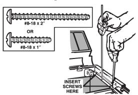
Hold the mounting bracket in place with the rod. Two sets of screws are provided. Use the short screws for flush bottom cabinets or the long screws for recessed bottom cabinets. Insert two (2) screws through the housing and into the mounting bracket. Do not tighten the screws completely.
