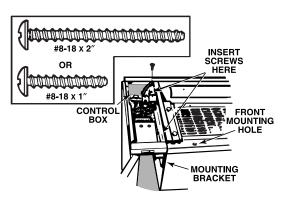
Insert two (2) screws, short or long as appropriate, through the control box and into the other mounting bracket. Do not tighten the screws completely.
