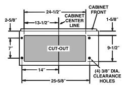
Prepare the cabinet bottom as shown above. Be sure to locate the cut-out and four holes from the front of the cabinet to ensure a flush mount.
