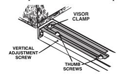
The visor slides each have a screw for adjusting the height of the visor trim, if necessary. The vertical adjustment screw allows the top and bottom edges of the visor trim to be matched with the control trim.
