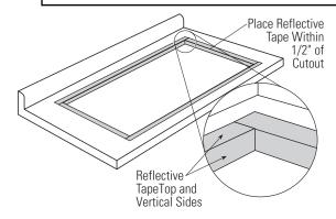
• Smooth rough edges of the cutout. Install reflective tape (supplied) to the opening, along the inside and 3/8" to 1/2" of the opening edge.
