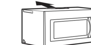
To vent through wall, see step C in installation section of manual.
