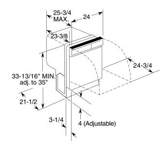
Countertop This wall area must be free of -90 90° pipes or wires 24" MIN. Electrical wiring is 3" from cabinet Hot water Electrical 34-1/2±1/4" Underside of countertop to floor line on wiring on left right Plumbing and electrical service must enter inside shaded area 19" MIN. from wal 24" From White (neutral) Ground Black (line) 24" MIN.
