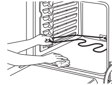
Gently lift the bake element Wipe up heavy soil on the oven bottom.
