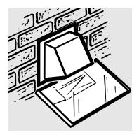
Check the inside of the exhaust hood with a mirror to rid of debris
