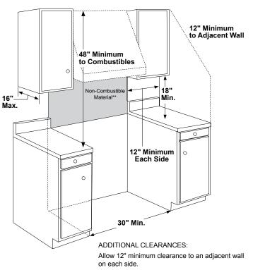
Working areas adjacent to the rangetop should have 18" minimum clearance between countertop and the bottom of the wall cabinet.
