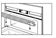
**Step 2:** Remove the front grille by taking out the 2 screws that hold it in place.
