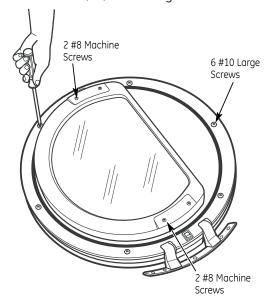
6. With the screws removed, turn the door over and separate the silver cover part of the door from the door frame and set aside.
