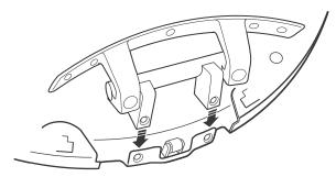
12. Loosely fasten the hinge assembly to the edge using 2 machine screws (#8).
