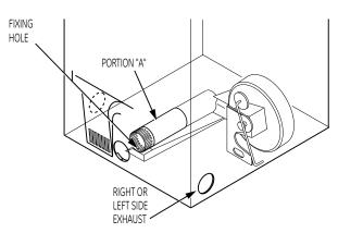
Reconnect the cut portion (A) of the duct to the blower housing. Make sure that the fixing hole is aligned with the tab in the base. Use the screw saved previously to secure the duct in place through the tab on the appliance base.
