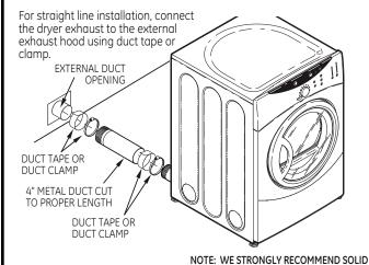
METAL EXHAUST DUCTING. HOWEVER, IF FLEXIBLE DUCTING IS USED IT MUST BE UL-LISTED METAL, NOT PLASTIC.
