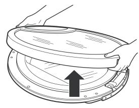
7. Unlock the 4 tabs on the plastic cover and separate theplastic cover from the frame.
