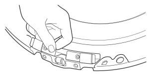
16. Secure the hinge cover with the 2 tapping screws (#8).
