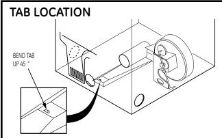
Through the rear opening, locate the tab in the middle of the appliance base. Lift the tab to about 45° using a flat blade screwdriver.
