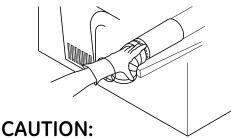
Internal duct joints must be secured with tape, otherwise they may separate and cause a safety hazard.
