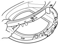
18. Place the outer door onto the inner door.
