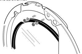
15. Place the hinge cover in position. Align the hinge cover holes with the holes in the door.
