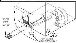
Detach and remove the bottom, right or left side knockout as desired. Remove the screw inside the dryer exhaust duct and save. Pull the duct out of the dryer.
