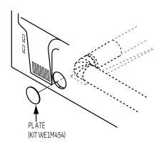
Connect standard metal elbows and ducts to complete the exhaust system. Cover back opening with a plate (Kit WE1M454) available from your local service provider. Place dryer in final location.
