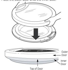
19. After reversing door, there will be a mismatch between the outer door and the inner door.
