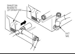
• Apply duct tape as shown on the joint between the dryer internal duct and the elbow.
