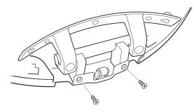
13. Hold the door on its side with one hand and fasten the remaining 2 screws as shown. Then tighten the 2 screws (#8) holding the hinge assembly.
