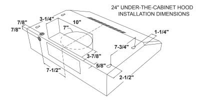
Exhaust outlet connects to  $3\text{-}1/4" \times 10"$  rectangular duct. Vent top or rear. Includes rectangular damper.
