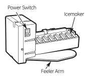
If ice cubes get stuck in the icemaker, set the power switch to **O** (off) and remove the cubes. Set the power switch to **I** (on) to restart the icemaker.
