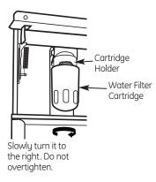
**IMPORTANT NOTE:** Remove the water filter to immediately stop any water leak from the Icemaker/Dispenser system. The water filter cartridge holder (bracket) acts as a cut-off valve when the filter is removed and will prevent further leaking.
