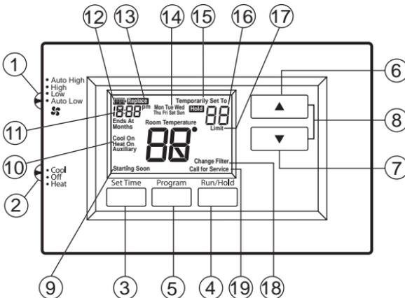
Whenever “ Replace ” appears in the display, new premium brand AA alkaline batteries should be installed. If the space will be unoccupied for an extended period and either “ ” or “ ” is displayed, install new batteries before leaving.
