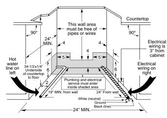
**Note:** Dishwasher must not be installed more than 10 feet from sink for proper drainage. All plumbing and electrical work must be in accordance with local codes.
