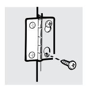
Remove the remaining screws from the side of the opening from which the door was removed. With these screws secure each hinge at the bottom. Tighten the two top screws of each hinge. Reinsert the plastic plugs on the side from which the door was removed.
