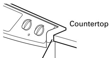
Make sure the edge of the countertop fits flush against the end of the front control panel
