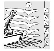
The oven has a special low shelf (R) position just above the oven bottom. Use it when extra cooking space is needed, for example, when cooking a large turkey. The shelf is not designed to slide out at this position.
