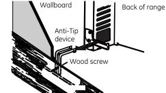
Install the sleeve anchor into the drilled hole and then install the lag bolt through the device. The bolts must be properly tightened as recommended for the hardware.
