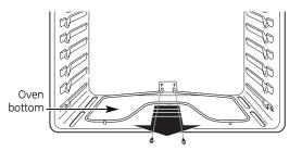
**D.** Lift the rear of the oven bottom enough to clear the lip of the range frame, push it back, and then pull it up and out.
