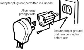
**CAUTION:** Attaching the adapter ground terminal to the wall receptacle cover screw does not ground the appliance unless the cover screw is metal, and not insulated, and the wall receptacle is grounded through the house wiring. The customer should have the circuit checked by a qualified electrician to make sure the receptacle is properly grounded.
