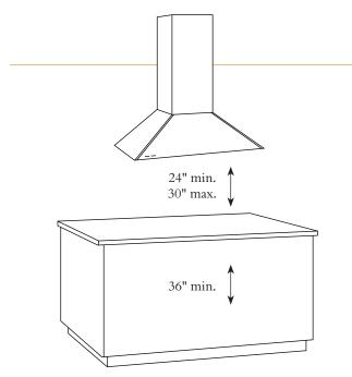
The exact installation height is determined by the ceiling height and duct cover trim strips provided with the hood. For optimum performance, the hood must be installed 24" min. and 30" max. above the cooking surface.
