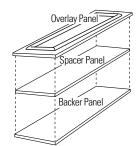
NOTE: Left-to-right offset is not always equal to top-to-bottom offset.
