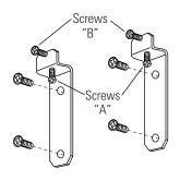
**Note:** Screws "A" and "B" are pre-assembled onto the brackets. Do not remove these screws.
