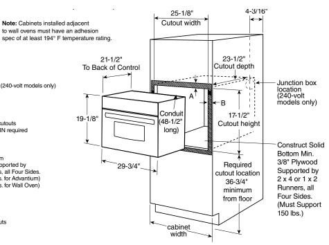
A=Allow 1" overlap of oven over bottom edge of cutout. B=Allow 11/16"-3/4" for overlap of oven over side edges of cutout.
