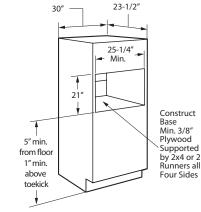
all models. The amount of overlap on the sides depends on the actual cutout width. Allow 1-1/4" case trim overlap on the top for models PSB9240 and for models ZSC2200, ZSC2201 and ZSC2202.
