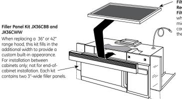
Filter Kit JX81J– Recirculating Charcoal Filter Kit To be used when the Spacemaker microwave oven cannot be vented to the outside.
