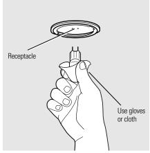
Push the bulb straight into the receptacle all the way. Then replace the screen.
