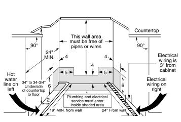
**Note:** Dishwasher must not be installed more than 10 feet from sink for proper drainage. All plumbing and electrical work must be in accordance with local codes.
