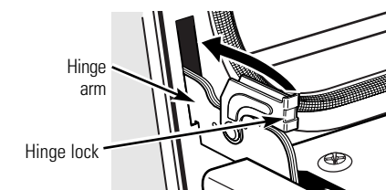
Push hinge locks up to lock.
