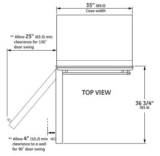
\*\* These refrigerators are equipped with a 2-position door stop. The factory-set 130° door swing can be adjusted to 90° if clearances to adjacent cabinets or walls is restricted. Allow a 15" minimum clearance to wall for pan removal. If the 90° door stop position is used, pan access is maintained, but pan removal is restricted.
