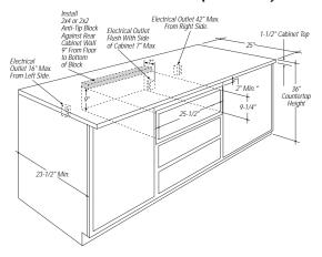
**Note:** When installing warming drawer with a cooktop, allow a 2" minimum from cooktop burner box bottom to top of cut-out.
