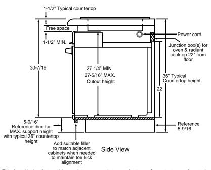
This installation is to achieve minimum gap between bottom of countertop and control panel. **Note:** For this installation, the bottom trim **will not** be flush with a typical 4" toe kick.
