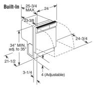
Important Note: GE kit number WD35M34 needed when adapting GE convertible dishwasher to a built-in installation. Contains built-in dishwasher water valve, hardware and complete instructions for changing a GE convertible dishwasher for underthe-counter installation.
