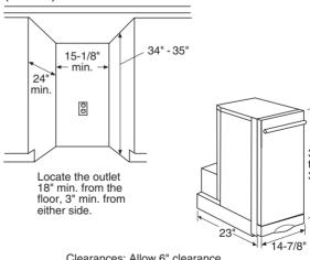
Clearances: Allow 6" clearance to a vertical wall on the right side for bag removal. Allow 23" at the front for a full drawer opening.
