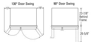
Allow minimum clearances for freezer door and fresh food door for a full 130° door swing and to allow for pan removal.
