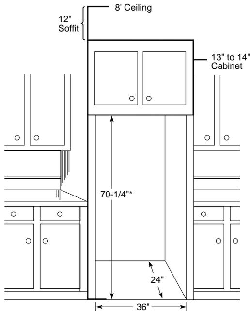
\*The rough-in dimension of 70-1/4" is minimum and is measured from the finished floor to top of opening (or the underside of the overhead cabinets). For Models with Trim Kit: If frameless style cabinets are planned for above the refrigerator, you may need to consider adding a maximum of 1/4" (70-1/2") to height of opening to allow additional clearance between cabinet doors and top of refrigerator trim when cabinet doors are in open position.
