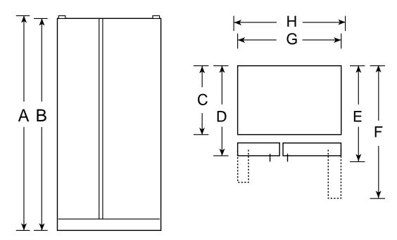
**Note:** If the doors cannot be fully opened because of an obstruction or a wall on either side, a door stop should be provided to prevent door or wall damage. If the doors cannot be opened at least 90 degrees, access to the drawers is limited.
