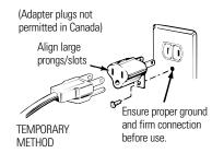
The larger slot in the adapter must be aligned with the larger slot in the wall receptacle to provide proper polarity in the connection of the power cord.
