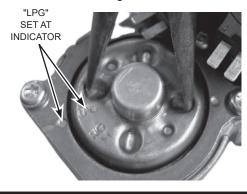
**8.** Using a 3/8" wrench, remove the NG burner orifice from the gas valve assembly turning it counterclockwise. Install the LP orifice from this kit.
