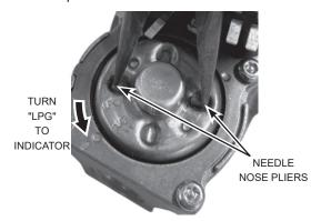
Rotate the dial counterclockwise, lining up "LPG" marking with the indicator on the gas valve.
