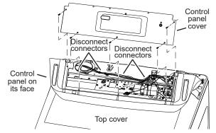
Disconnect the connectors from the control board and set the control panel aside.
