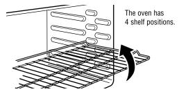
To remove a shelf, pull it toward you, tilt the front end up and pull it out.
