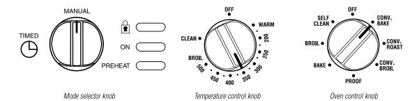
Single oven controls shown set for convection baking.
