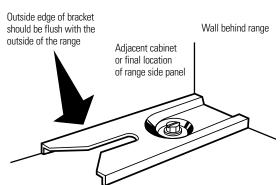
Screw the bracket securely to the floor with the screw provided. The screw is self-drilling in wood, plywood, particle and chip board, and most metal framing. If attaching to masonry, you can buy suitable screws and/or anchors at hardware stores. Use a masonry drill to drill the required holes.
