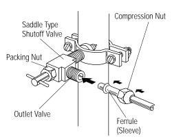
• Turn on the main water supply and flush debris from the line. Run about a quart of water through the tubing into a bucket. Shut off water supply at the shut-off valve.
