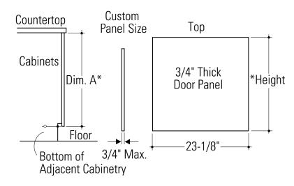
The custom panel should be constructed in the same manner as cabinet doors. All edges can be seen and must be finished for the best appearance.
