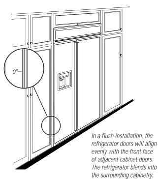
Monogram built-in refrigerators can be installed flush with typical 24-3/4" deep cabinetry.
