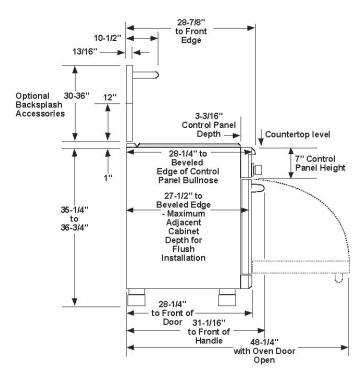
12" min. to combustibles or 0" to a non-combustible material above the cooking surface
