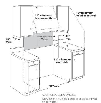
Working areas adjacent to the rangetop should have 18" minimum clearance between countertop and the bottom of the wall cabinet.
