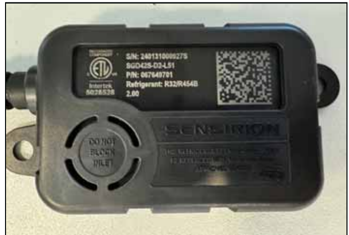
FIGURE 14. Example of Clear, Unobstructed Sensor Inlet
